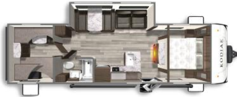
280BHS - Length: 32' 10" Weight: 5,519 lbs Fresh Water: 44 gals. Grey Water: 39 gals. Waste Water: 28 gals.
