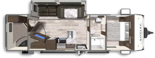
296BHS - Length: 33' 11" Weight: 6,070 lbs Fresh Water: 44 gals. Grey Water: 78 gals. Waste Water: 28 gals.
