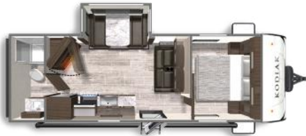
242RBSL - Length: 28' 10" Weight: 5,137 lbs Fresh Water: 44 gals. Grey Water: 39 gals. Waste Water: 28 gals.
