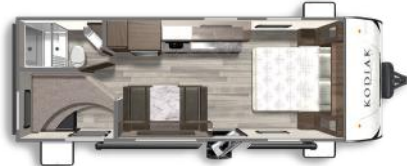
220BHS - Length: 26' 11" Weight: 4,157 lbs Fresh Water: 44 gals. Grey Water: 39 gals. Waste Water: 28 gals.
