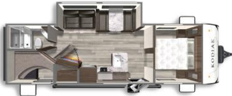
270BHS - Length: 31' 10" Weight: 5,336 lbs Fresh Water: 44 gals. Grey Water: 78 gals. Waste Water: 28 gals.
