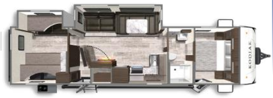
332BHS - Length: 37' 3" Weight: 7,157 lbs Fresh Water: 44 gals. Grey Water: 78 gals. Waste Water: 28 gals.
