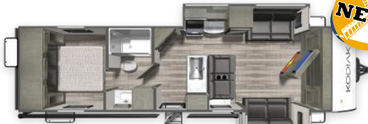
310FLSL - Length: 35' 9" Weight: 6,910 lbs Fresh Water: 44 gals. Grey Water: 78 gals. Waste Water: 28 gals.
