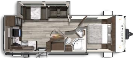
257RKS - Length: 29' 11" Weight: 5,562 lbs Fresh Water: 44 gals. Grey Water: 78 gals. Waste Water: 28 gals.
